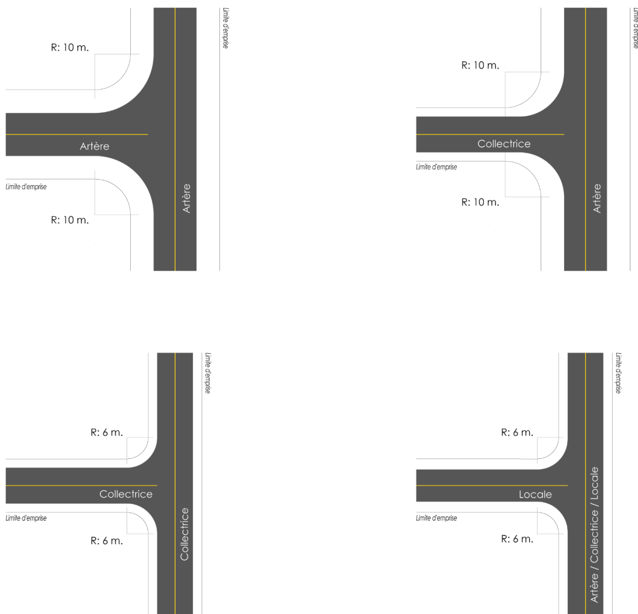
Figure IX : Conception des raccords des intersections
